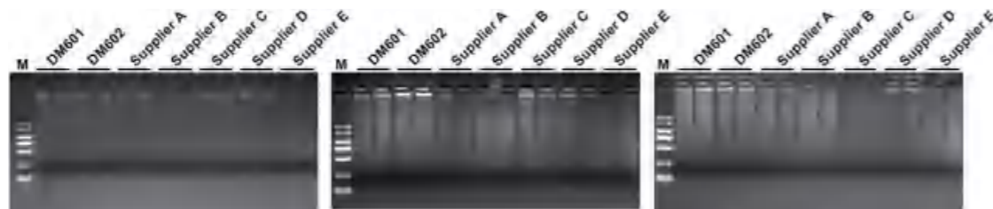
Figure 1. DNA Gel Electrophoresis Images for Vazyme #DM601/#DM602 and Suppliers A - E for 30 mm2 Mouse FFPE Sections (Lung/Liver/Spleen)
