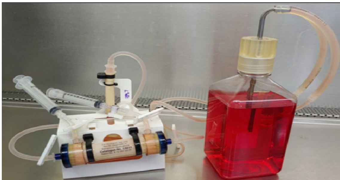
Figure 4: The FiberCell hollow fiber bioreactor is a completely closed system providing protection for the cells from microbial contamination and protection for the operator when working with infectious pathogen
